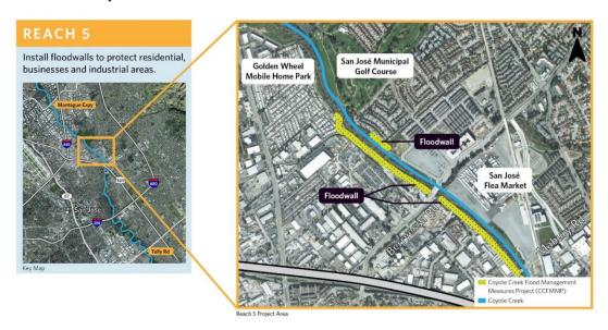
In Reach 5, two of the floodwalls are approximately 2,300 feet long each and the third floodwall is approximately 300 feet long.
