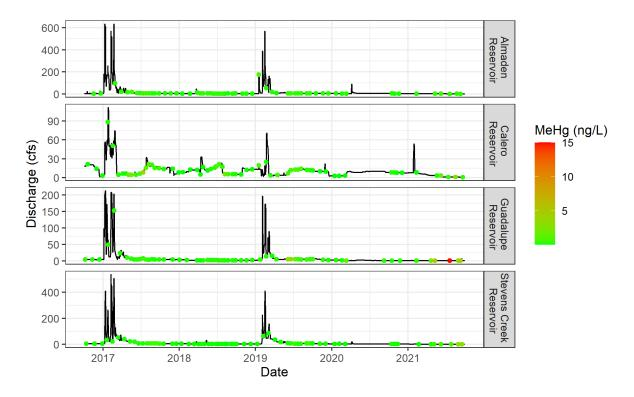
Figure 27: Hydrograph of outlet flow and measured MeHg concentrations at Almaden, Calero, Guadalupe, and Stevens Creek reservoirs.
