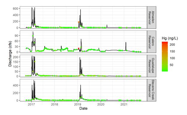
Figure 26: Hydrograph of outlet flow and measured total Hg concentrations at Almaden, Calero, Guadalupe, and Stevens Creek reservoirs.
