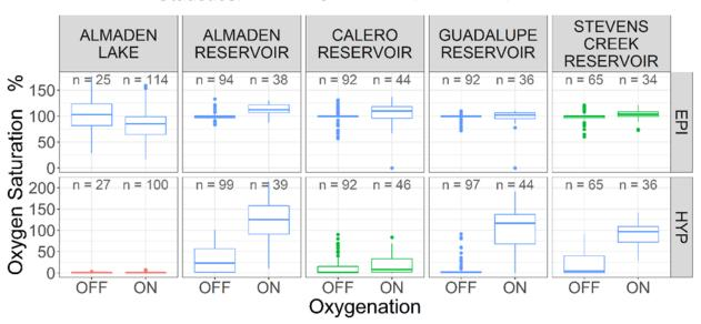
Figure 7: Epilimnetic and hypolimnetic dissolved oxygen saturation before (OFF) and during (ON) seasonal operation of the treatment systems.
