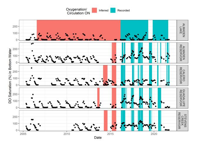
Figure 3: Hypolimnetic dissolved oxygen saturation in reservoirs and Almaden Lake.
