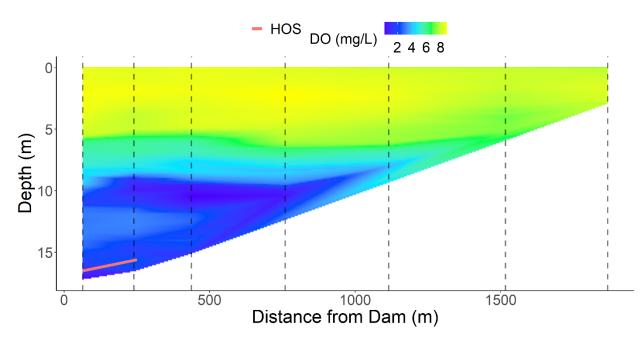
Figure 9: Lateral extent of hypolimnetic oxygenation in Calero Reservoir (September 3, 2021). The extent of the diffuser line is shown in red.
