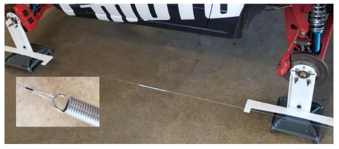
Place the loop ends of two braided cables around the hooks at the end of a spring and position the spring in the middle between the stands on one side of the car.
