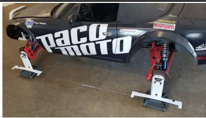
Thanks for choosing our Alignment Hub Stands for your chassis setup needs. We hope you'll find them as handy, accurate, and easy to use as we do! Each stand has a max capacity of 1000 lbs, and fits both 4 and 5 lug vehicles with 12 or 14mm lugs, bolt patterns from 4x95.25 to 4x114.3, 5x100 to 5x130, and a hub center max diameter of 72.5mm. They will fit just about every vehicle under a 4000lb curb weight!
