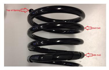
Repeat the first two steps and work the second piece down to the second coil. Make sure the spiral material overlaps as shown. Do these same steps to the other rear spring.
