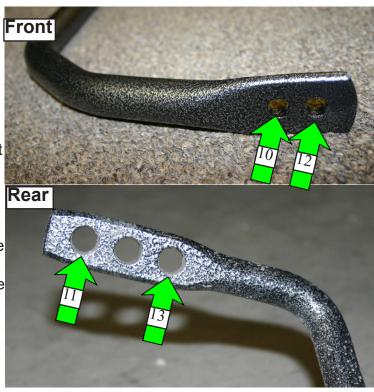
the car's handling. Most people are more comfortable (and safer) with a car that understeers slightly. As a starting point, use the holes farthest ends of the bar on the front bar (10) and the middle holes on the rear bar.
