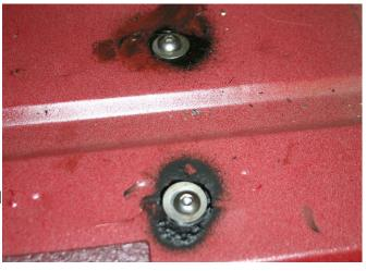
bolt - this ensures good alignment. Drill the rest of the holes, spray some undercoating, install the remaining bolts with anti-sieze on the threads, and then tighten them slowly (to prevent galling) - you may see the floor start to deform slightly. Be careful when drilling beside the fuel and brake lines. They can be gently pulled out of the way while
