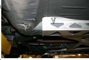
both rails up equally before drilling any holes in the floor pan. It is very important to get both sides square so that if you're adding the Butterfly section (available as a package or separately) it will bolt directly up.
