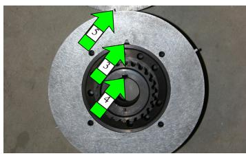
4. 36-2 tooth timing wheel only: The 36-2 tooth wheel should have "FM" legible from the front (6, backwards from the back). If you don't know what a 36-2 tooth wheel is, you don't have one. Be sure that the notch in the wheel (7) lines up with the keyway (8).
