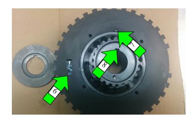
5. Slip the spacer over the toothed gear, and tighten it down - be sure to use blue Loctite (242) here. Slip the rearmost flange back into place. Be sure to line up the roll pin appropriately.
