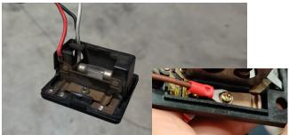
the same way as dash light. Attach the provided small eyelet (36-80045) to the end of the brown wire. Remove the screw from the dash light switch plate. Be careful as the plate, switch, and screw are all small and easy to drop. Reinstall the screw through the small eyelet and back into the switch plate (image shows the eyelet installed on a dome light to demonstrate what it should look like). Installing the screw too tightly can cause the switch to feel stiff.
