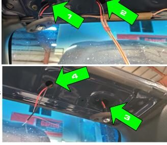
and the single red wire into the red side of the butt connector. Properly crimp and heatshrink the connections. Repeat this to connect the brown and black wires.
