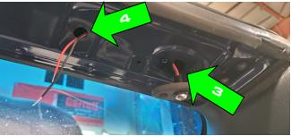
10. Feed the wire ends of second LED light assembly through the visor hole on the passenger side (3) and pull the wires down through the adjacent hole inboard (4).
