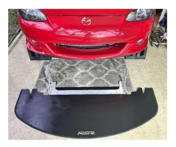
4. Before bolting the splitter, the factory hardware must be removed from the mounting points. Remove the bolts that hold the factory undertray and both bolts for the sway bar Bracket. These are 10mm bolts. Bolts to remove pictured below.
