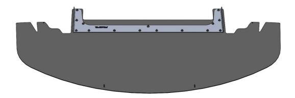
2. Now it's time to bolt the mounts. To do this you will use the 6 provided M6x16 hex bolts and hex nuts. Put together one mount, each take 3 bolts and nuts, hand tighten them together (they have to be loose enough so they can be adjusted later in the car). To put these together you will need a 10mm socket and a 10mm wrench. Once put together the mounts should look like this:
