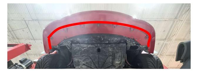
5. Now it's time to bolt the splitter up. Put it (the splitter) under the car, it is easier if you have help from somebody but if you do not you can use a jack to lift it and get it into position.
