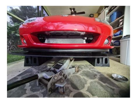
Once the splitter is in position it can be bolted in, use the 6 provided M6x25 hex bolts along with the M6 washers to bolt it. Hand tighten the bolts for the meantime as some height adjustment may be required. Do this for both sides. Once the mounts are bolted in, they should look somewhat like this:
