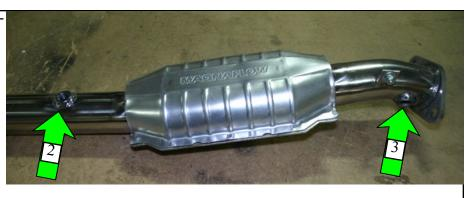
it should be plugged, there is no use for it. Do not install a wideband O2 sensor behind the catalytic converter, as the accuracy of the wideband is diminished when it's installed behind the catalytic converter. The bung in front of the catalytic converter is provided for a wideband O2 sensor. Widebands are only relevant for cars with programmable engine management.
