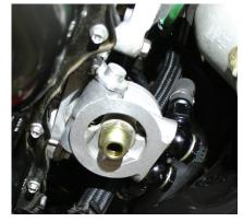
hold it in place. Tighten this to 107-141 lb-**IN**. Install the oil filter and tighten it to the same torque. If this is a new filter, be sure to smear some oil on the O-ring on the top of the oil filter and pre-fill the filter before installing.
