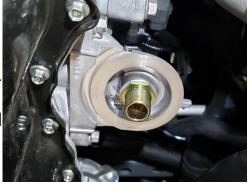
supplied union and factory hose clamps. Use zipties to keep the hoses from being in contact with sharp or abrasive objects. Using the supplied 12mm Allen tool removed the adapter holding the factory cooler in place (9). Install the supplied fitting with the shorter threads installing into the engine plate and tighten to 107-141 lb-IN.
