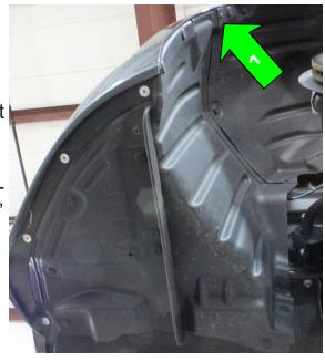
3. Remove the center fabric splash pan. There are two 8mm head bolts on the front edge, eight 10mm head bolts (three on each of the upper sides, two in the rear), and two plastic fasteners at the rear. Pay attention to how the front edge overlaps the bumper cover for installation. The plastic fasteners are different than the wheel well fasteners but their centers still pull out the same distance.
