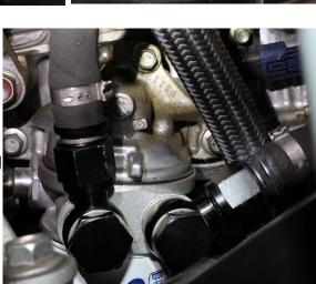
rearward fitting on the thermostat. Be sure to oil the faces (tapers) and threads of the fittings before installing. Tighten the hoses to 29 lb-ft, or hand-tight plus one turn. The forward hose should be at roughly 2 o'clock, the rearward hose should be around noon. Tighten the banjo bolts to no more than 29 lb-ft.
