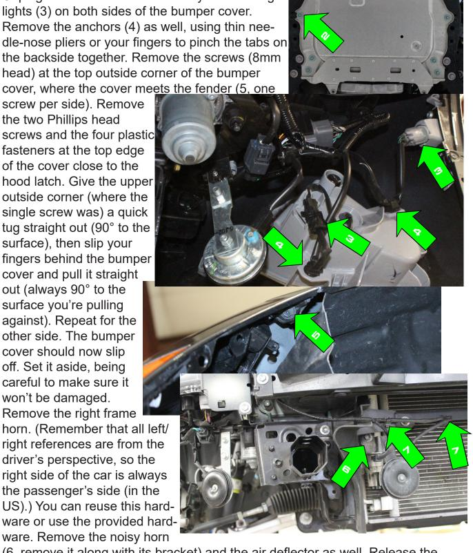
(6, remove it along with its bracket) and the air deflector as well. Release the two anchors for the horn wiring (7) and let the horn hang for the time being. The air deflector won't be reinstalled.
