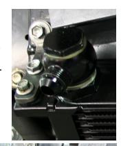
11. Smear some oil on the rubber gasket on top of the oil thermostat and slip it onto the threaded stud for the oil filter. Route the hoses as you're slipping the oil thermostat into place. Try to route them such that there will be as little rubbing as possible, but it's impossible to avoid all of it. Be certain to carefully orient the thermostat such that it clears the oil filter base on the engine and sits perfectly flush. Use the gold adapter that's included with the thermostat to
