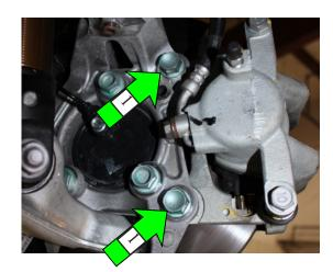
3. If you're replacing the rotor, remove the old one (this kit works with stock rotors). If your rotor won't come off, thread an M8x1.25 bolt into the threaded hole on the face of the rotor. It should pop off of the hub once you thread it in a little way. Thoroughly clean the new rotor with brake cleaner (oil / grease will destroy pads), then slip it onto the studs.
