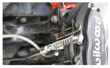
17. Adjust the cable at the lever (in the cabin) as needed (9). There should be about 3 clicks before you feel resistance, but be sure that the cable is loose at the caliper when the parking brake isn't engaged. Don't forget to replace the heat shield from step 12.
