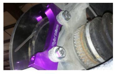
8. Be sure the rotors are clean of any oil, then install them. Slotted rotors do have a left and right, install them appropriately. They should be labeled, but if not, install them as shown in the picture - this is the right (passenger) side of the car. The calipers shouldn't be in place yet.
