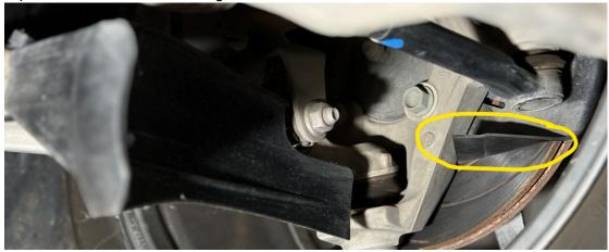
2.9. For increased airflow trim approximately one-third of the wheel wind shield to enhance airflow to the brake cooling deflectors. Alternatively, you may remove the wheel wind shield entirely.
