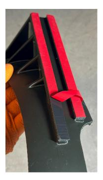
2.6. Stick the deflector to the front lower control arm as illustrated in the picture below, ensuring there is sufficient clearance from the shock absorber base, as indicated by the green marking.
