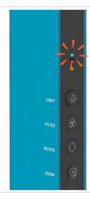
Once the white LED stops blinking, the amber LED will turn on and the VZ-X should disconnect automatically from your computer indicating a successful update. You can now reconnect to the VZ-X and sign back into the Advanced Settings Page to verify that the firmware version has been updated to VZ-X\_2033.
