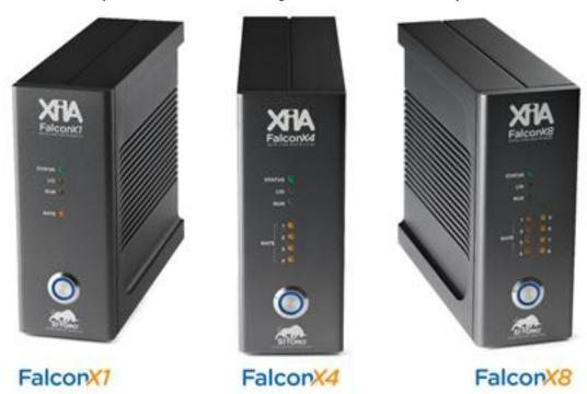
Power is provided to the FalconXn by an external, medical-grade 12V, 5A power supply. Communication is through a high-speed gigabit Ethernet connection. SMA connectors are used for the analog inputs. Several MCX connectors are used for digital control inputs; finally, a high-density connector is used to provide 32 digital I/O lines.
