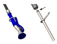
Step 2: Apply plumber's tape to top of riser threads and attach to spring assembly. Tighten with wrench.
