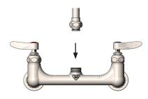
Step 4: Grab riser assembly and lower the EasyInstall® endfitting into faucet body. Press down until the endfitting "pops" in.
