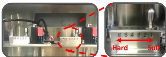
The viscosity adjustment, located behind the faceplate, controls the firmness of dispensed product. The higher the viscosity, the more firm the product. Viscosity settings should NOT need continuous adjustment.
