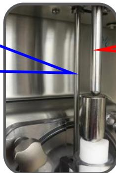
Arm moves up and down and tells machine when product is being dispensed.
