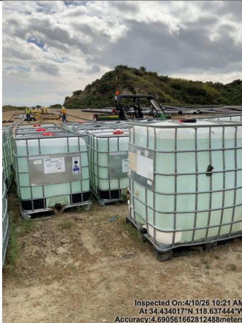
Photo 48 Sodium hypochlorite totes stored outdoors without secondary containment
