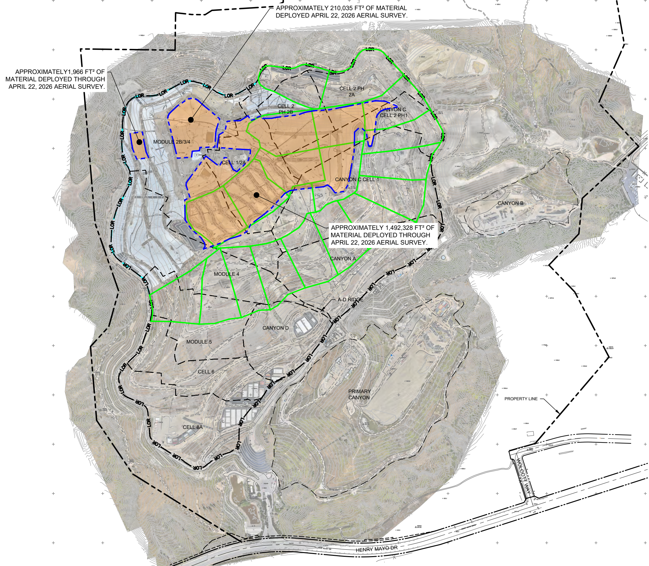
FIGURE 1 APPROXIMATE LIMITS OF DEPLOYED EVOH GEOMEMBRANE CHIQUITA CANYON LANDFILL CASTAIC, CA
