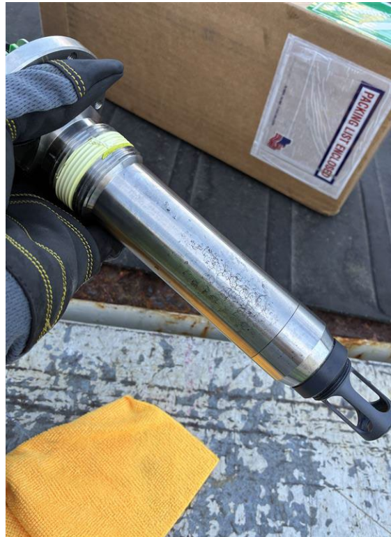
Pilot 3 - CH4/CO2 Probe missing Cover
