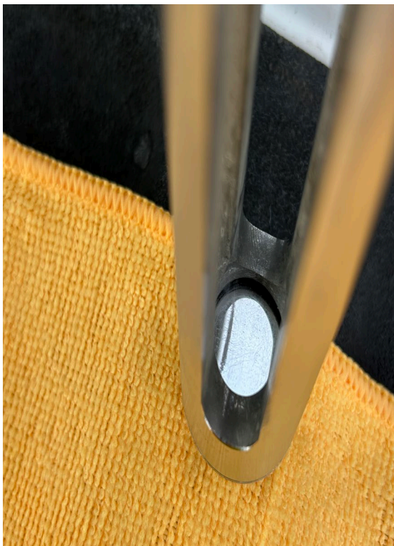
Pilot 4 - Water line on O2 Sensor Optic
