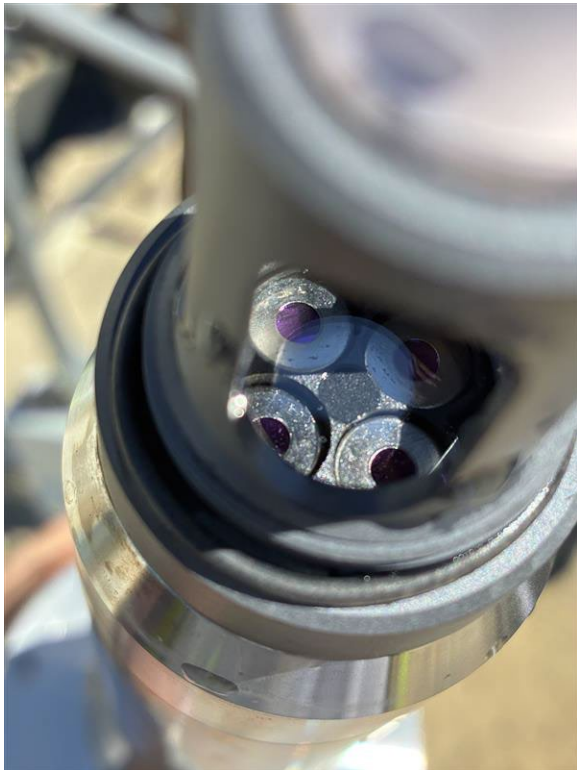
Pilot 2 - CH4/CO2 Probe Sensors
