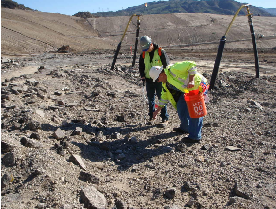
Photo 4.1 Typical Field Screening to Determine Flux Chamber Sampling Locations.
