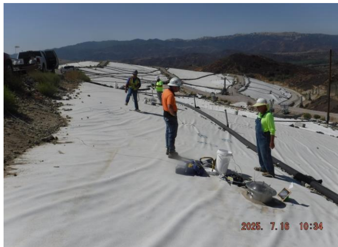
Photo 1.2 Flux Chamber on Membrane Covering Portion of Landfill.
