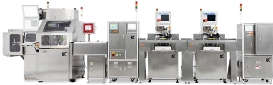
Figure 10.7: In-line System composed of a die-bonder, snap cure oven, and other assembly equipment for CMOS image sensor packages. Courtesy of Kulicke and Soffa Industries.
