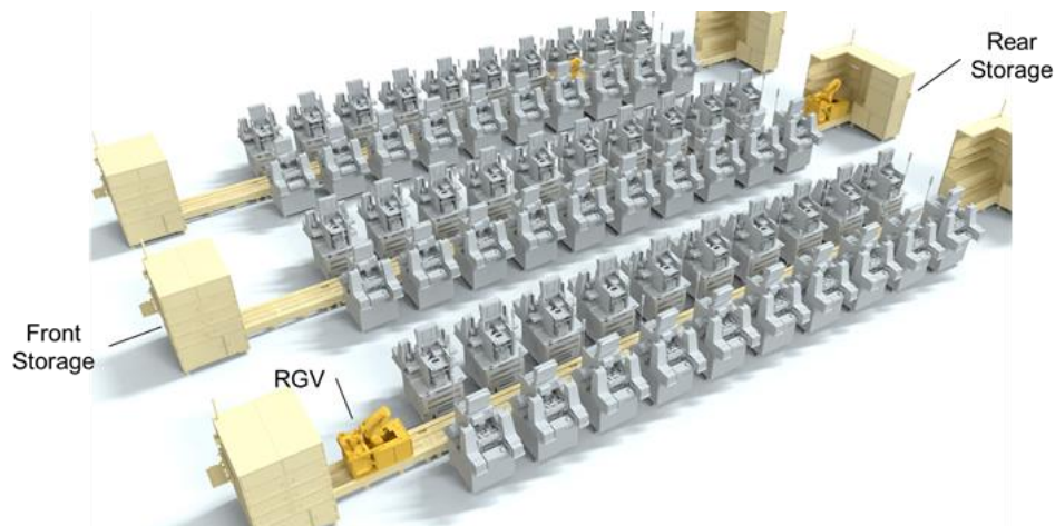
Figure 10.6: Rail Guided Vehicle Servicing Wire Bonders. Courtesy of Kulicke and Soffa Industries.
