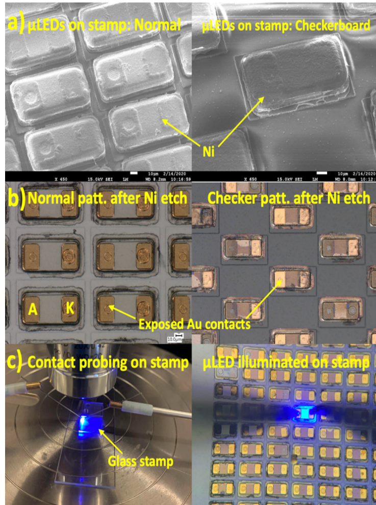
Figure 4.6. (a) SEM image of as transferred microLEDs sitting on glass stamp (face up); (b) Optical image of microLEDs with exposed contacts after removal of Ni layer and seed; (c) Contact probing of microLEDs on stamp confirming successful operation [1].
