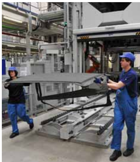
Carbon fiber panels are pressed into shape.
