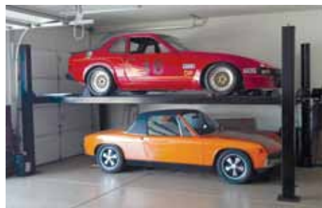
The American Custom Lifts Voyager four-post lift will fit in a bay of a two-car garage.
