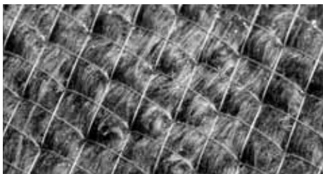
This close up shows the carbon fiber mat woven from the tow produced in Moses Lake.
