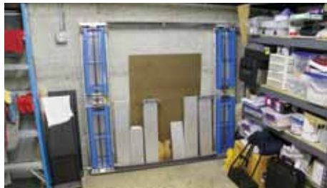
The entire EZcarlift system can be stored flat against a wall. The photos also show the drive-over ramp set.
