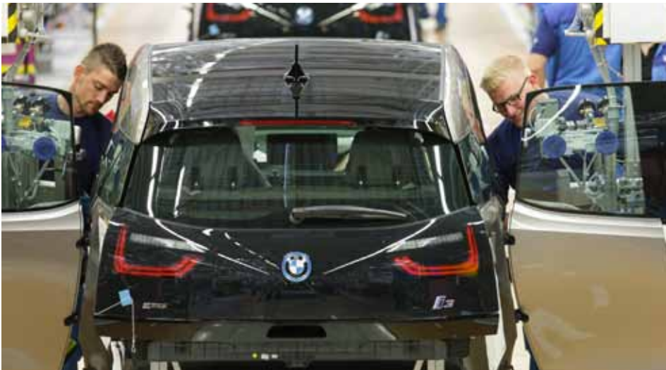
An i3 in assembly with some of the plastic exterior panels in place.
