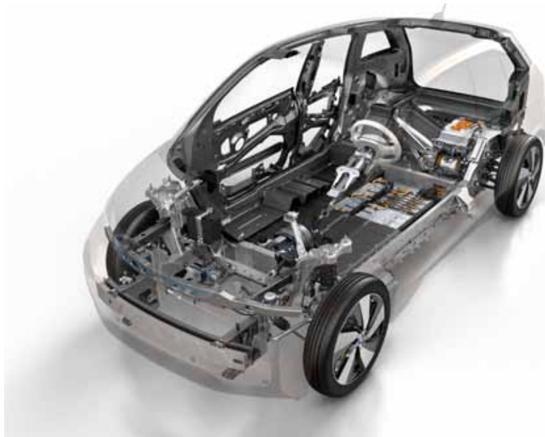
The batteries sit low in the chassis, providing a low center of gravity.
