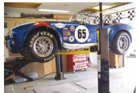
The MaxJax 2 post carlift will easily fit in a single bay of a two car garage.
