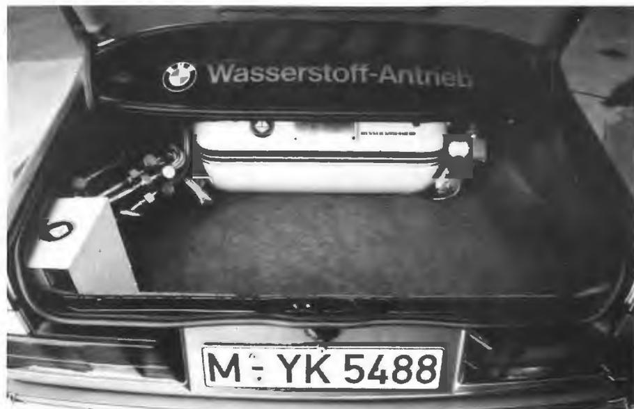
Development of a viable hydrogen vehicle concept is a task for automotive researchers, and it is primarily this challenge that BMW's researchers have taken on. Recent BMW development efforts have been concentrated on a 735iL sedan, powered by a modified version of that model's 3.5-liter six-cylinder engine with a relatively simple external air-fuel mixing system.
