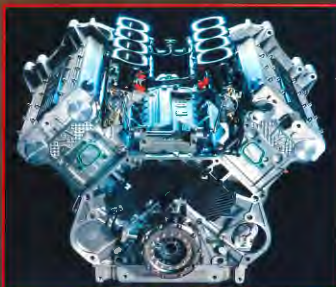
The 600hp V8 'customer racing engine' specifically designed for US racing series.
