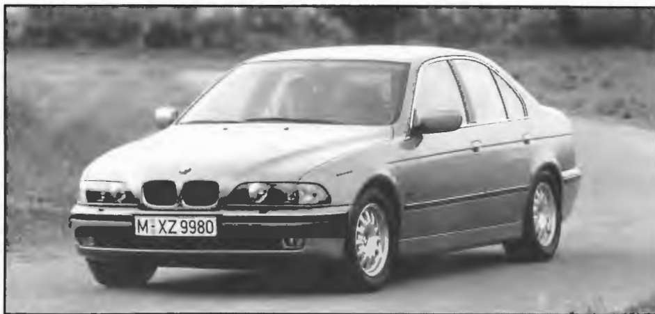
The kidneys raise with the hood. the hood creases merge with the A-pillar.
