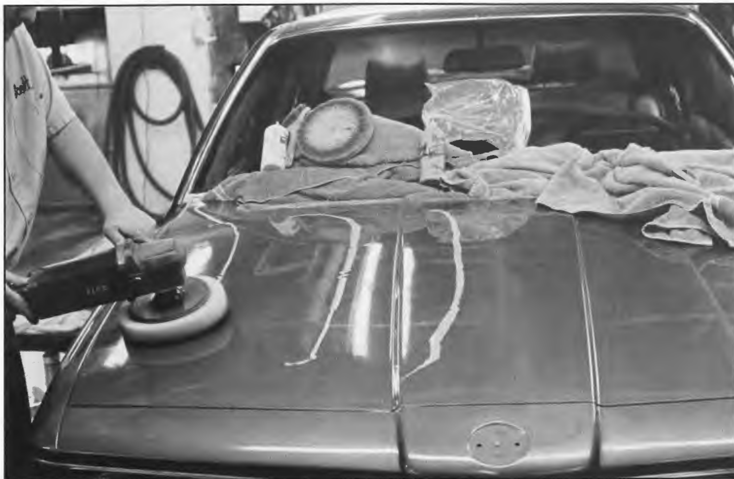
Photo 5. Move the buffer in straight strokes, lengthwise along the car, picking up the liquid along the way.
