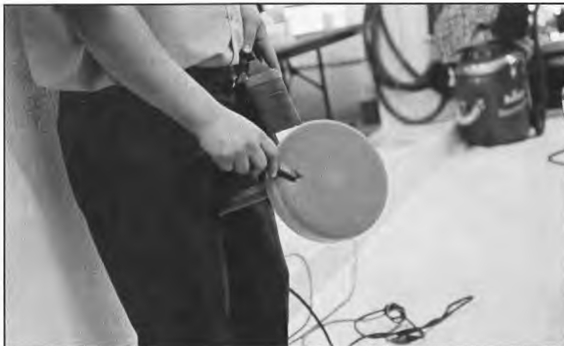
Photo 3. Cleaning the wheel with a plastic brush.
