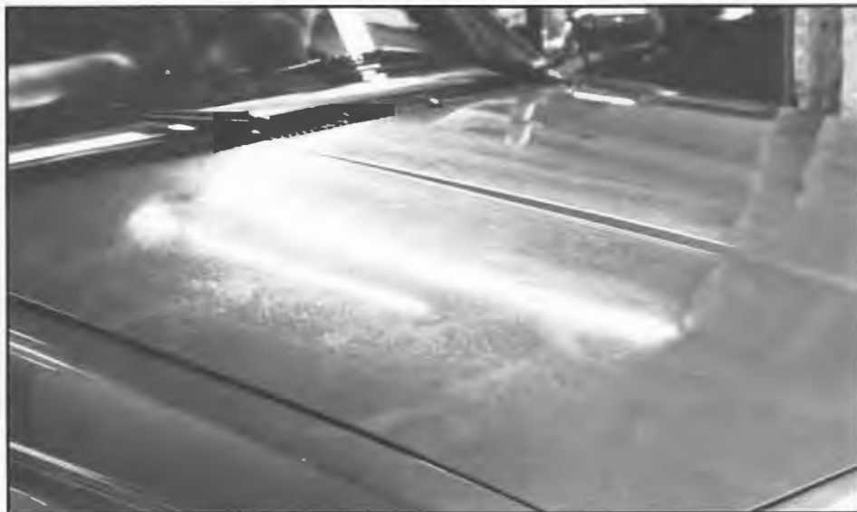
Photo 1. Classic clear coat failure. No amount of polishing can correct this — it needs repainting!
