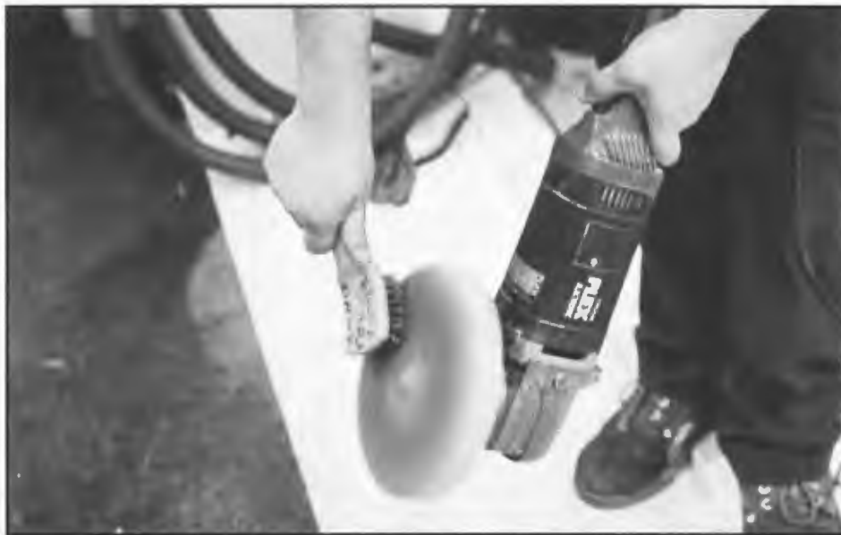
Photo 4. Trimming the wheel with a steel brush.
