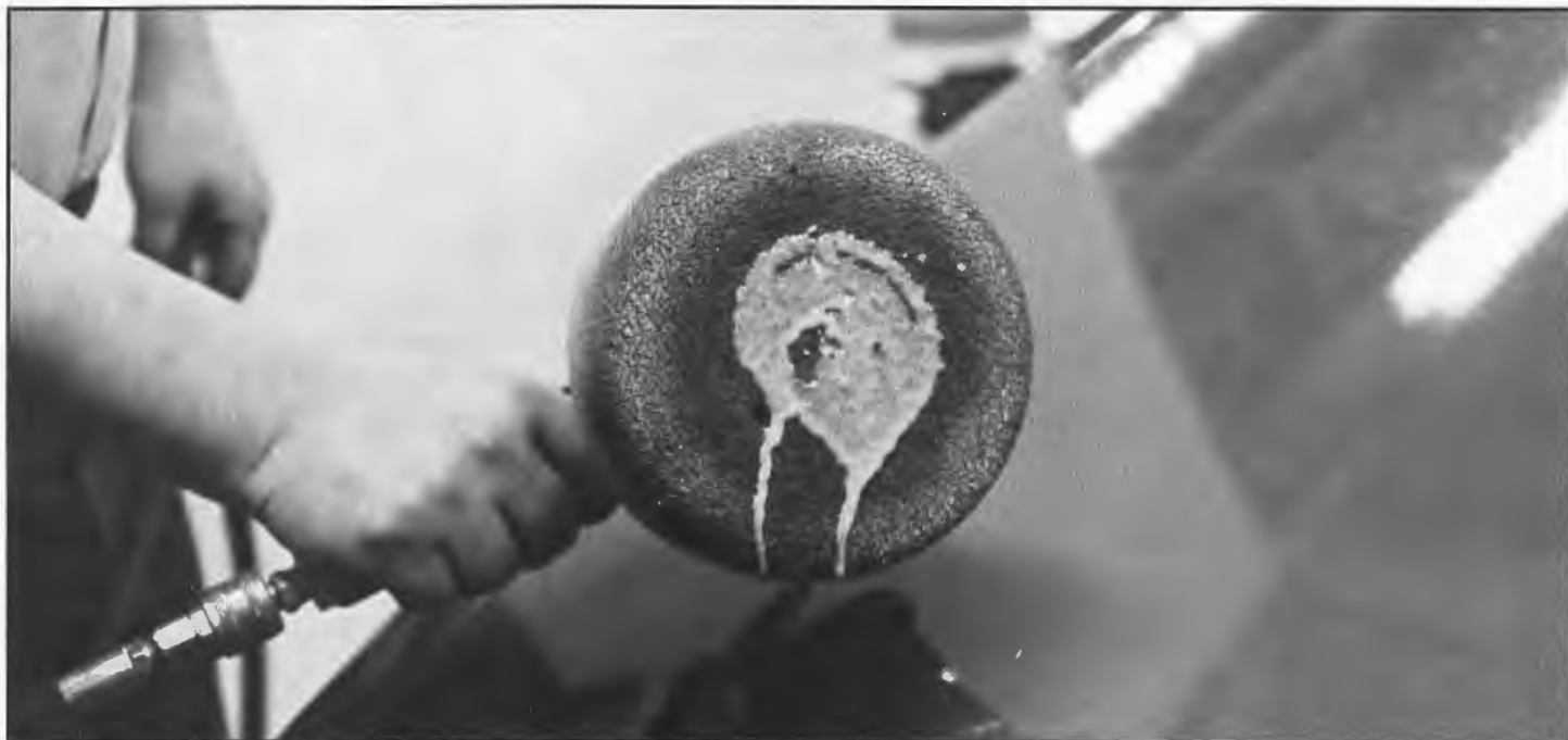
Photo 6. Applying Meguiar's material to a polishing pad on a hutch.
