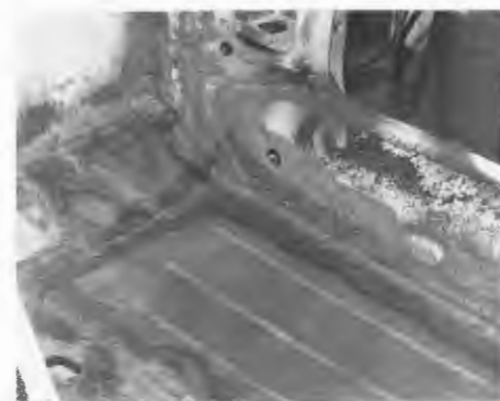
New sheetmetal is welded in and prepared for primer.
