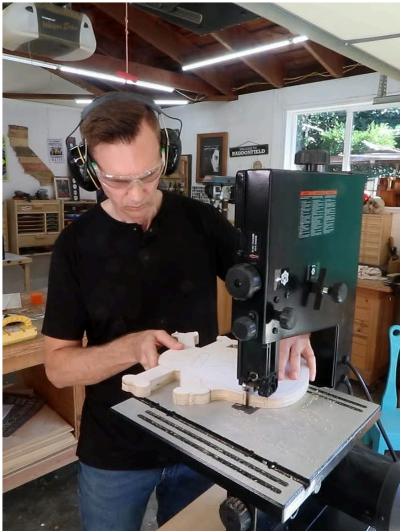
Cutting tight curves.
