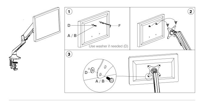
Step 4 Install the monitor to the plate
